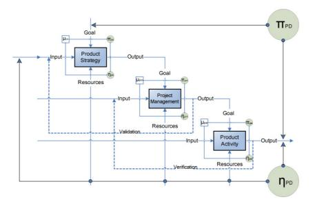
Figure 2. The proposed PDOPM model with the three generic levels of activities: product strategy, project management, and product activity. The relations of uncertainty ( $\mu$ ), effectiveness (II), and efficiency ( $\eta$ ) are also shown in the figure, both for each activity and for the complete PD process.
