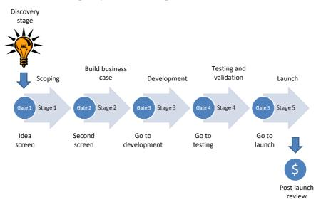
Figure 2. The generic Stage-Gate process [1].
