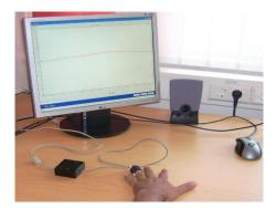
Fig. 1. Taking finger temperature measurement using a temperature sensor
