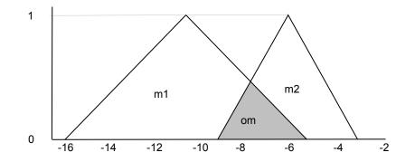
Figure 21. Fuzzy similarity using triangular membership functions. X-axis denotes the feature values and Y-axis degrees of membership functions.
