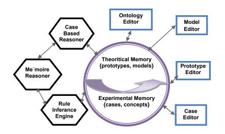
Figure 24. Me'moire architecture. Right: memory acquisition tools, left: reasoning components. Adapted from [6].
