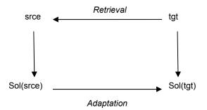
Figure 23. The CBR in KASIMIR. A source case (srce,Sol(srce)) similar to tgt is retrieved from the case base and adapted to solve tgt.
