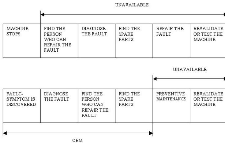
Figure 1: Differences in run-to-failure technique and CBM.
