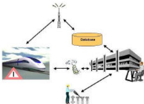
Figure 4: The communications between the rail vehicle, maintenance centre and service centre.
