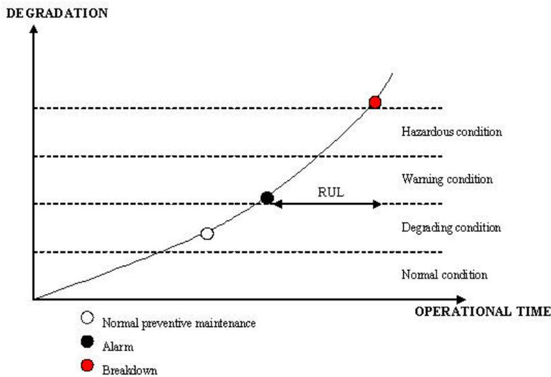
Figure 2: The normal preventive maintenance is often carried out before the component, sub-system or system is showing any signs of fault. With the CBM technique one often say “If it ain’t broke, don’t fix it”. RUL is an abbreviation of Remaining Useful Life.
