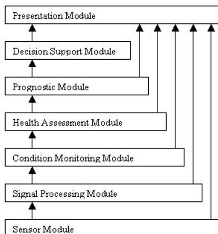
Figure 3: The seven layers in OSA-CBM standard proposal.
