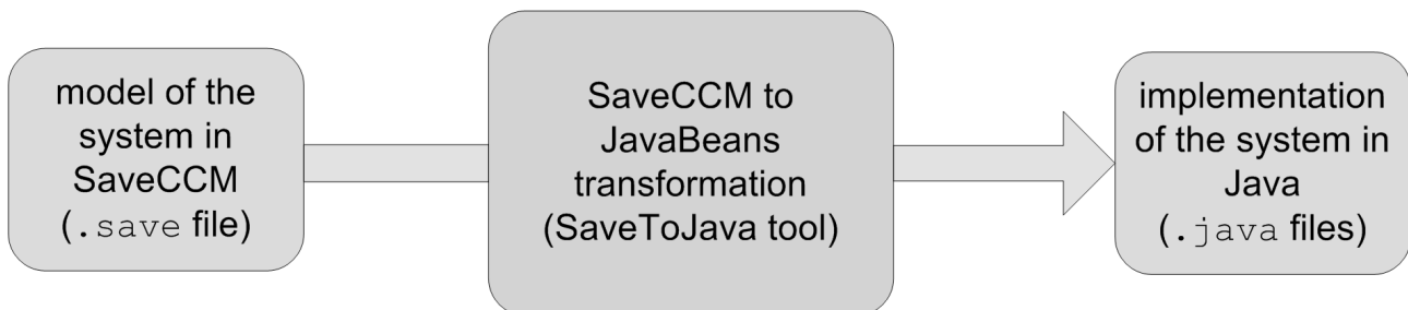
Figure 5.1: Transformation from SaveCCM to JavaBeans
