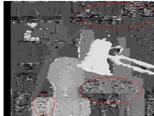
Figure 7.2: The areas with the most noise (red circles) have low-texture and/or low signal-to-noise ratio.
