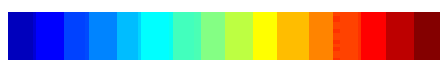
Figure 6.3: The colormap for the disparity images. Blue indicates a small disparity, and red a big disparity.
