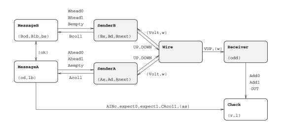
Figure 5: Philips Audio-Control Protocol with Bus Collision.
