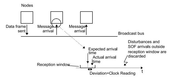
Figure 3: Exchange of Clock Readings.
