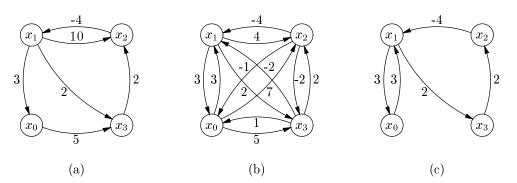
Figure 3: Graph for E (a), its shortest-path closure (b), and shortest-path reduction (c).
