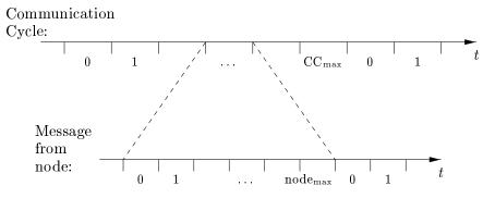
Figure 1: The Cyclic Operation of DACAPO.
