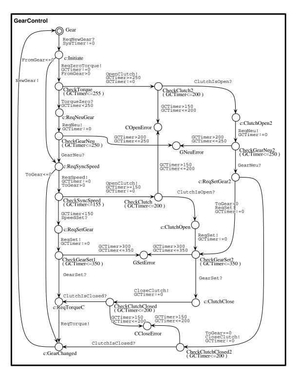
Figure 7: The Gearbox Controller Automaton.
