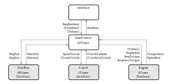
Figure 4: A Flow-Graph of the Gearbox System.
