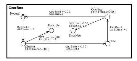
Figure 5: The Gearbox Automaton.
