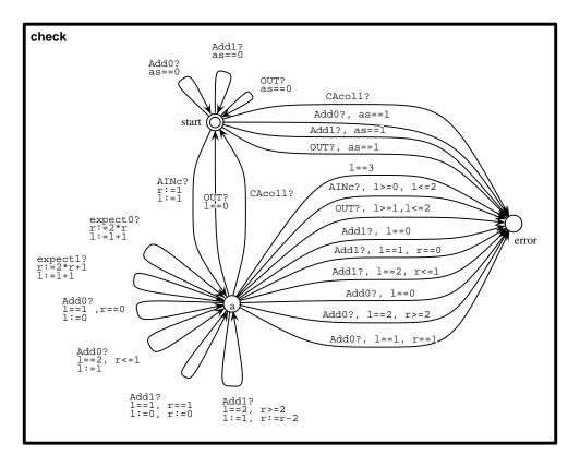
Figure 7: The Check Automaton.
