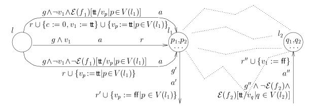
Figure 3: Illustration of a modified timed automaton  $\mathcal{M}(A_i)$  of  $A_i$ .
