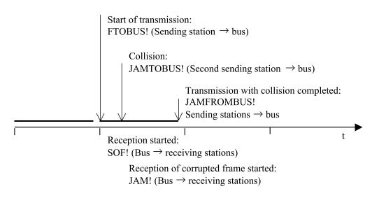
Figure 6: Message Transmission with Collision.
