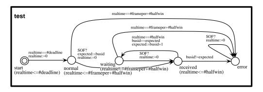
Figure 7: Test Automaton Used to Express Correctness Properties.
