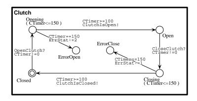
Figure 8: The Clutch Automaton.
