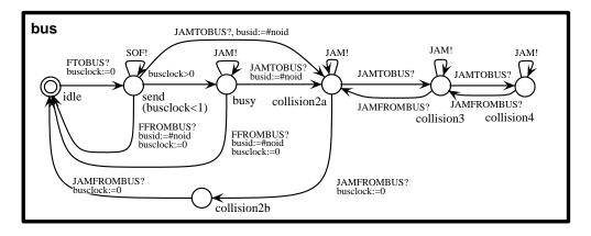
Figure 4: Timed Automaton Describing the Bus.
