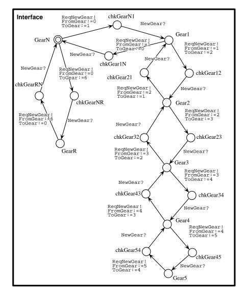
Figure 9: The Interface Automaton.
