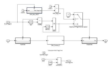
Fig. 5: Simulink pattern for modeling event-trigged execution of an EAST-ADL function with execution time. The block FMU\_function\_F represents the FMU.
