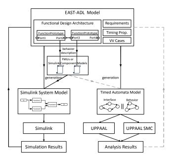
Fig. 2: Our simulation and model-checking methodology.
