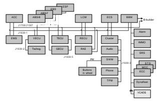
Figure 2. Volvo FH electronic architecture.
