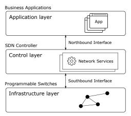
Fig. 1: SDN Architecture separates a network into tree layers: Application, Control and Infrastructure layer.
