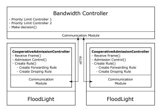
Fig. 6: Overview of the collaborative admission control using DART framework.
