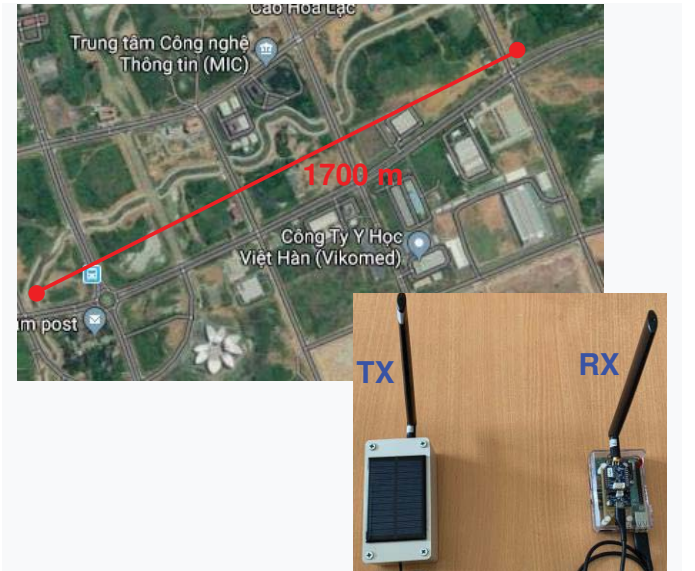
Fig. 4. The demonstrated monitoring system using proposed temperature Beat sensor and LoRa communication protocol.
