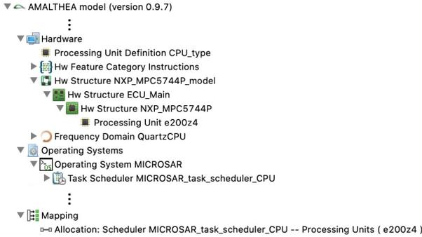
Figure 8: Extract of an AMALTHEA architecture depicting a `ProcessingUnit` element, a `TaskScheduler` element and the `SchedulerAllocation` element.
