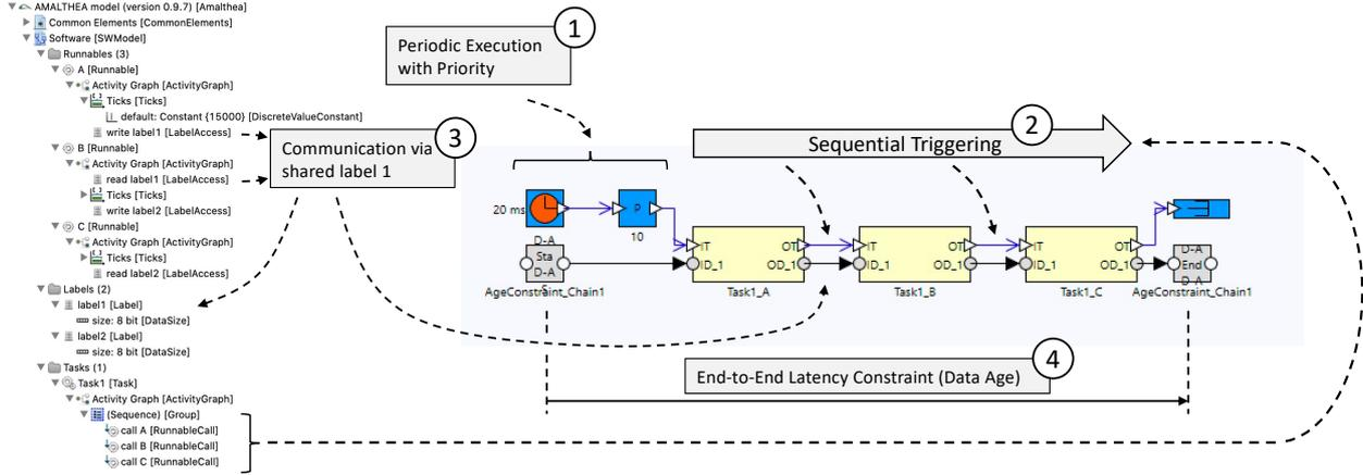
Figure 10: Extract of an AMALTHEA architecture and its RCM representation. Highlighted are the periodic execution with fixed priority (marking 1), mapping of runnable execution from AMALTHEA tasks to sequential execution in the RCM model (marking 2), communication via shared labels in the AMALTHEA model and mapping to communication via data channels in the RCM model (marking 3), and representation of end-to-end timing constraints in the RCM model (marking 4).
