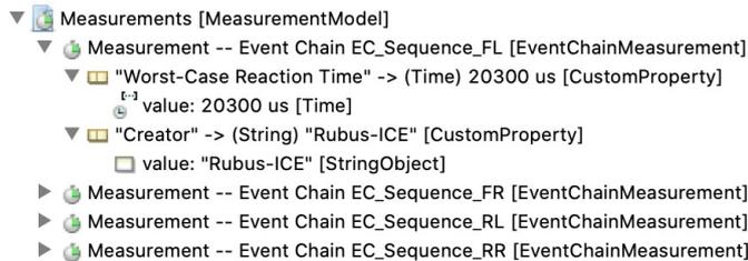
Figure 12: Extract of an AMALTHEA architecture depicting the back annotation of latency constraints.
