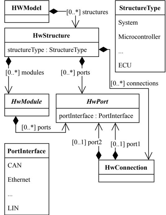
Figure 2: Simplified representation of the AMALTHEA hardware model.
