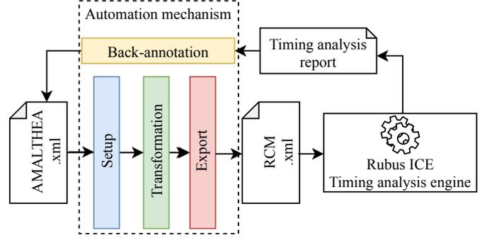
Figure 13: Overview of the automation mechanism and its phases.
