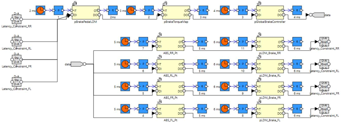
Figure 19: Excerpt of the RCM architecture of the BBW system created manually from a software engineer.
