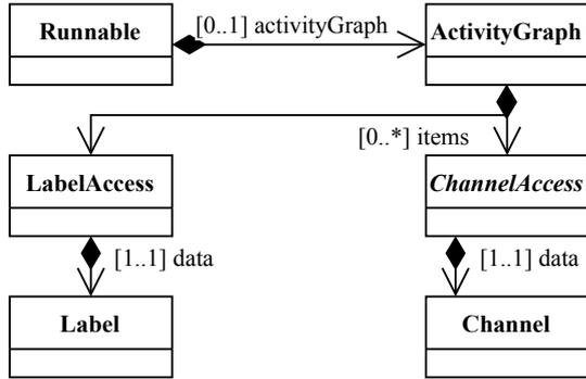
Figure 3: Simplified representation of the relationships among Runnable, Channel and Label elements.
