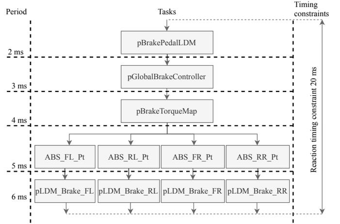
Figure 14: Block diagram of the BBW application. Different tasks and their communication pattern are shown. Task period and reaction time constraints are annotated.
