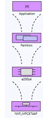
Figure 9: Extract of an RCM architecture depicting a `Partition` element, a `Core` element and a `Node` element.
