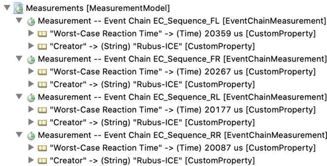
Figure 18: Excerpt of AMALTHEA architecture showing the back-propagation of the analysis results.
