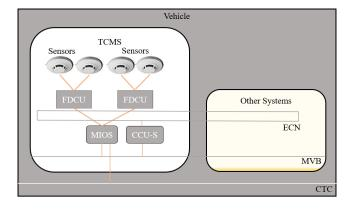
Figure 2: Architecture illustration of fire detection subsystem of TCMS
