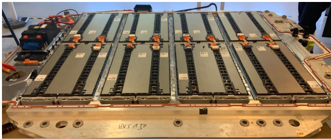
Fig. 2: An example of an EV battery pack after the lid and the connection cables have been removed. It contains 8 modules.
