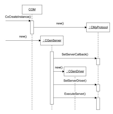
Figure 5-8 Call sequence to set up connections
