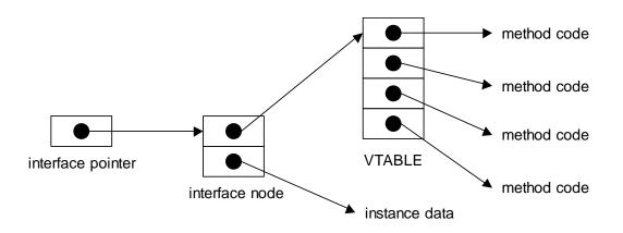
Figure 4-1 Typical format of COM interface nodes
