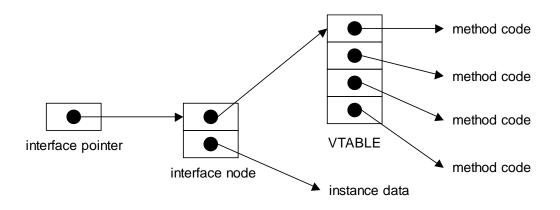
Figure 7-1 Typical format of COM interface nodes
