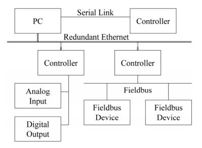
Figure 5-4 Example control system configuration
