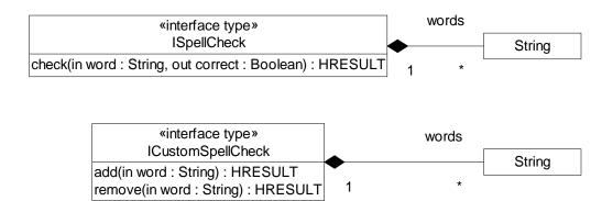
Figure 3-3 Example interface specification diagram
