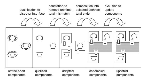
Figure 2-6 Reference model for composition of software components
