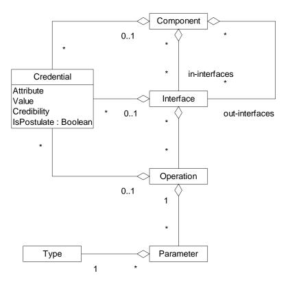
Figure 3-7 UML metamodel of concepts used to specify extra-functional properties of software components
