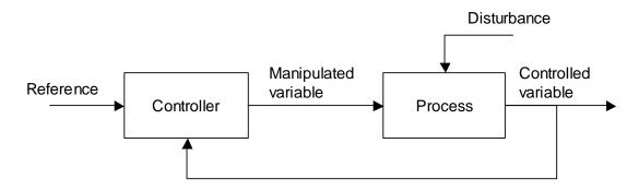
Figure 2-9 Closed-loop control system
