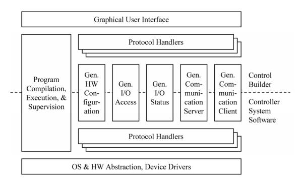
Figure 5-5 Component-based software architecture
