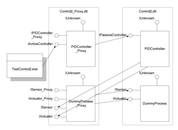
Figure 6-5 An application using a controller component with services
