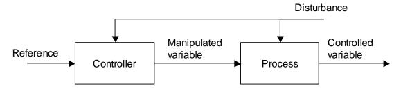
Figure 2-10 Open-loop control system
