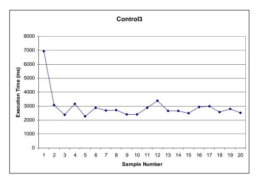
Figure 7-11 Measured initialization times for Control3
