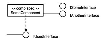
Figure 3-5 Component specification showing an interface dependency
