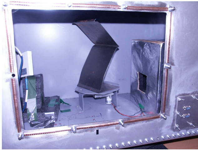
Figure 1. A small SFC with a shielded anechoic box with apertures.
