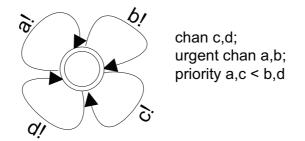
Figure 2: The automaton used for synchronization.
