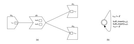
Figure 15: (a) Graphical representation of *connecting message ports to a message channel* and (b) its formal semantics
