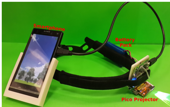
Figure 3. A photograph of the hardware device, equipped with a smartphone, a battery and a pico projector. The housing for both items is in-house 3D printed.
