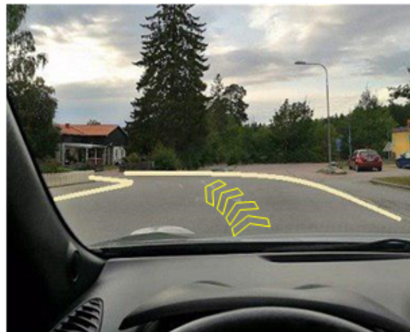
Fig. 2. An example of AR information on Head Up Display.
