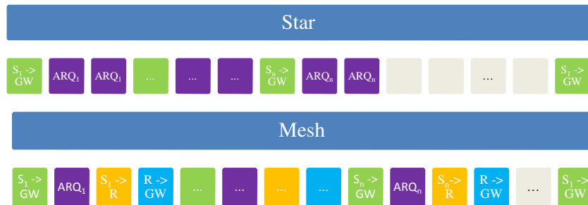
Fig. 2.3. Example of time slot allocation for the star (upper) and mesh (lower) networks
