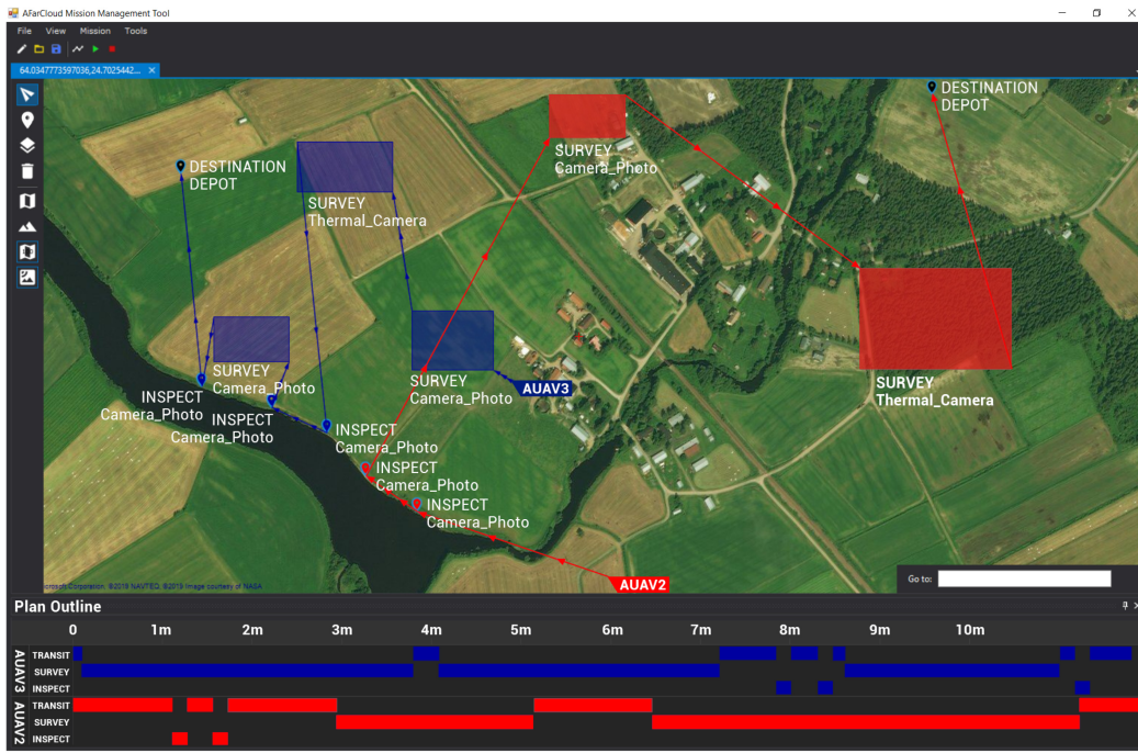
Fig. 2. Screenshot of the GUI with a generated mission plan and a plan outline in a form of a Gantt chart.
