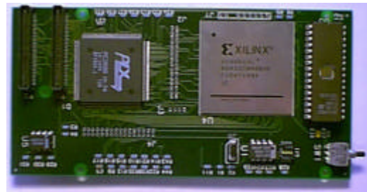
Figure 4: Picture of a RTU-PMC board
