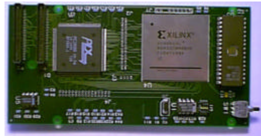
Figure 4: Picture of a RTU-PMC board
